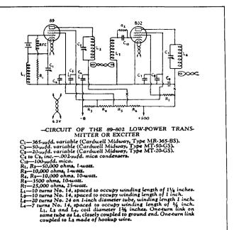
fig. 4. This two-tube, 10-meter transmitter of 1936 is modern enough to do a good job on the band today. The 802 pentode amplifier is capable of 40 watts input. A 7-MHz crystal was used. Cathode circuit of the 89 oscillator tunes to about 10 MHz to provide correct feedback. Plate circuit is tuned to 14 MHz, and 802 is a frequency doubler to 28 MHz. (Drawing reproduced from the January, 1936, issue of QST.)
